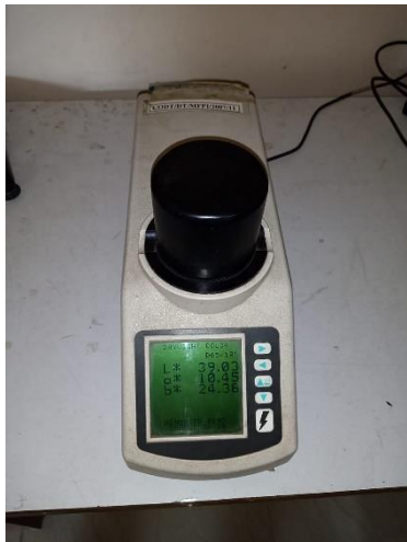
Fig-5 Measurement of colour by Hunter colour Lab colour-flex calorimeter
