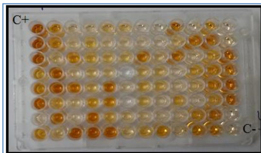
Fig-3 Microtitre plate showing the results of I-ELISA for detection of Brucella antibodies. C+ (Positive control), C- (Negative control) and Rest of the well: Field serum samples.
