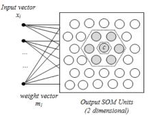
Fig. 2- A graphical representation of the SOM architecture with a 2D hexagonal grid
