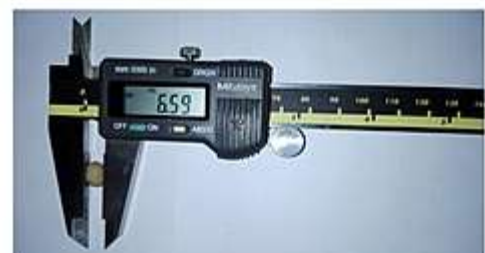
Fig-5b Thickness of pelleted seeds measured by digital Vernier calliper
