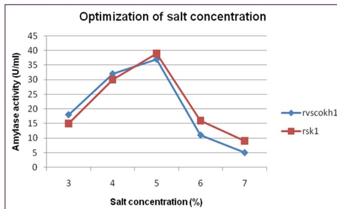
Fig. 3- Effect of salt concentration on enzyme activity in strain rvscokh1 & rsk1
