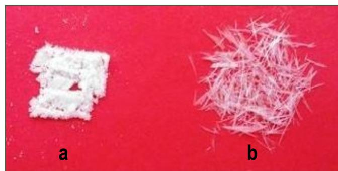
**Fig. 5-** Recrystallization of Gentamicin Sulfate USP. In the left is powder met the USP test specifications. In the right is the regular acicular crystal. These needles were collected from the three derivatization samples of 4 and 8 mg/mL each after being stored in 4°C overnight, filtered by gravity and air dried.
