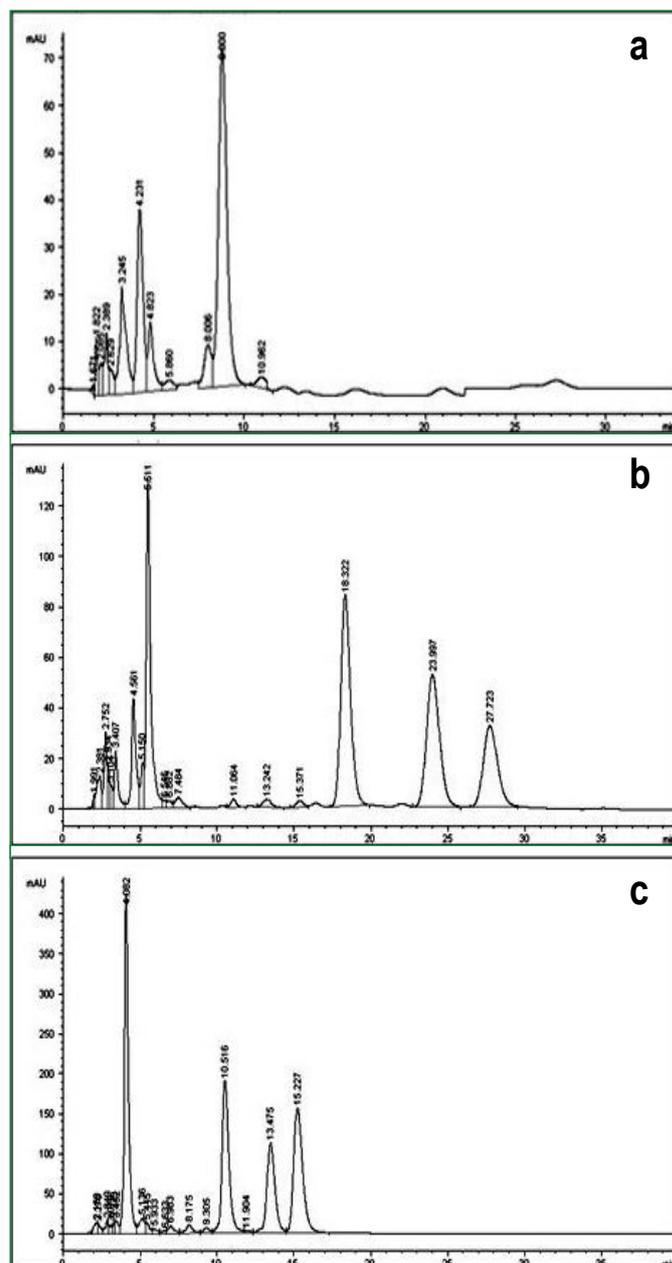
**Fig. 2-** The chromatograms of the first two study LC columns: (a) Aqua C<sub>18</sub>, (b) the Nuc leosil C<sub>18</sub> at the concentration of 2 mg/mL. The sample in chromatograms a) and (b) was prepared from the gentamicin sulfate powder met the USP test specifications, but eluted through an Aqua C<sub>18</sub> and a Nuc leosil column, respectively. Figure (c) was the chromatogram of the commercial Gentamicin Sulfate for Injection USP eluted by a Nuc leosil C<sub>18</sub> column.
