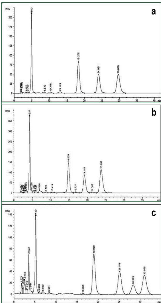
**Fig. 3-** The chromatograms of the third columns, Luna C<sub>18</sub>. Figure (a) was the sample prepared from the USP Gentamicin Sulfate RS and Figure (b) was the commercial Injection USP. Both displayed three aminoglycoside peaks. Figure (c) was the sample prepared from the gentamicin sulfate powder met the USP test specifications. All concentrations were at 2 mg/mL.
