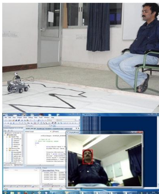
Figure 4: (a) Above: Robot tracking the face. (b) Below: Output of the tracker on the computer screen
