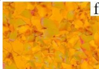
Fig. 1(f) Microphotograph showing Smectic-F phase (220X).
