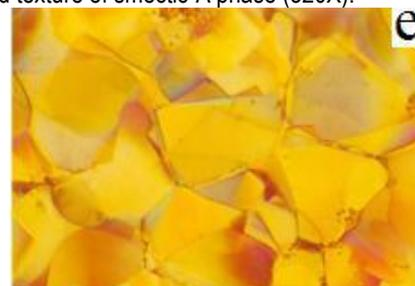
Fig. 1(e) Microphotograph showing Smectic-I phase (220X).
