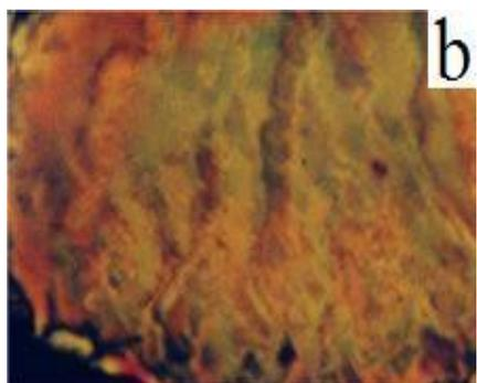
Fig. 1(b) Microphotograph showing Hexagonal grid pattern of TGB-A phase (360X).
