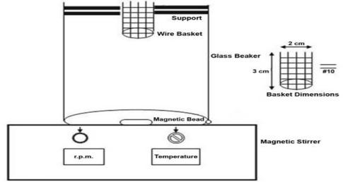
Fig. 1- Schematic representation of the disintegration test apparatus
